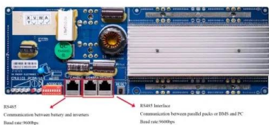
RS485 Communication between battery and inverter Baud rate:9600bps RS485 Interface Communication between parallel packs or BMS and PC Baud rate:9600bps
