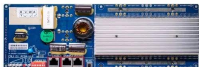
RS485 Communication between battery and inverter Band rate:9600bps RS485 Interface Communication between parallel packs or EMS and PC Band rate:9600bps
